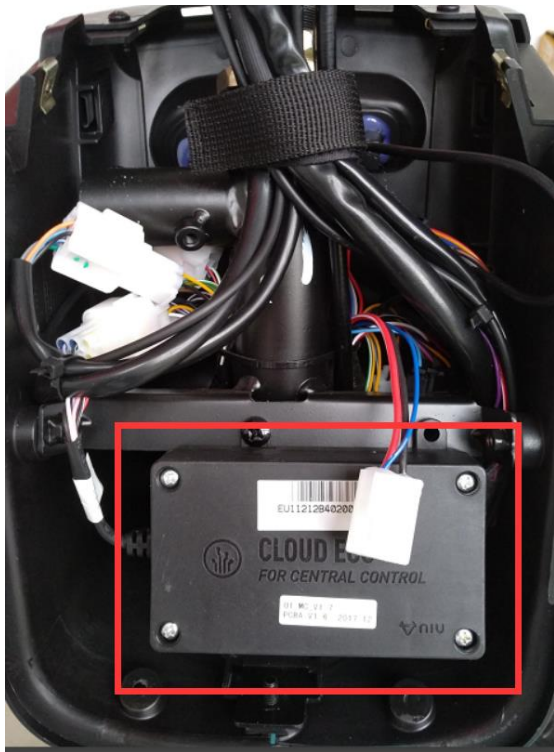
ECU connectors between main harness and ECU side
