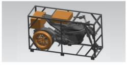
Remove the tightening belt of the vehicle, take out the accessory carton, the front fender carton, and the front tire assembly. 3
