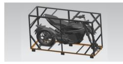
Remove the M6×12 hexagon flange bolts used for fixing at the lower part of the packaging frame to remove the upper part of the packaging frame.
