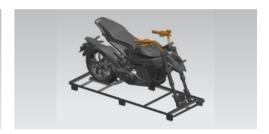
Adjust the angle of the handlebar, and then tighten the bottom four M8×25 hexagon socket head cap screws with a torque of 15~22 N·m.
