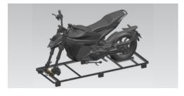
Take out the Φ12×193 front wheel axle, and remove the lower part of the packing frame.
