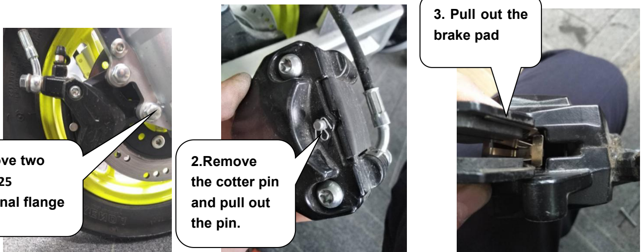
Pic 33. Remove the bolt
