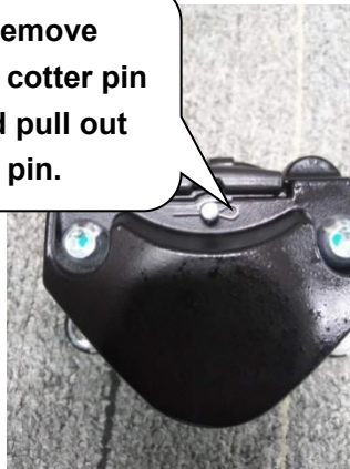
Pic 38. Remove the bolt Pic 39. Remove the cotter pin and remove the pin Pic.40. Pull out brake pads
