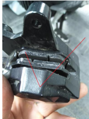
Pic 36. The brake pads are not installed properly, dangerous! Pic 37. Brake pads installed in place
