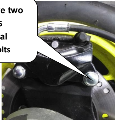
Pic 38. Remove the bolt Pic 39. Remove the cotter pin and remove the pin Pic.40. Pull out brake pads
