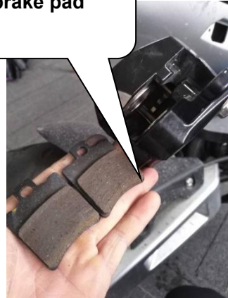
Pic 38. Remove the bolt Pic 39. Remove the cotter pin and remove the pin Pic.40. Pull out brake pads
