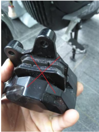
Pic 36. The brake pads are not installed properly, dangerous! Pic 37. Brake pads installed in place
