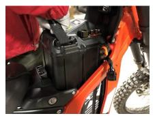
Step 2: Open the front battery plate
