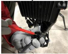
Step 2, black probe insert to the black wire port, red probe insert to the yellow, green and blue wire port, measure the voltage, normal voltage should between 4.5-4.7V
